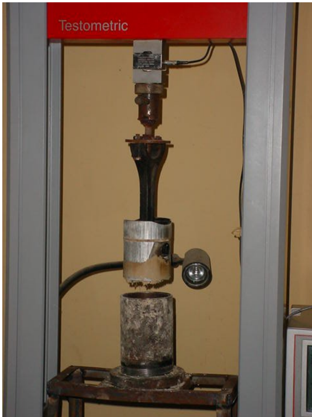
Figure .1: Showing the Piston-Cylinder assembly on the Universal Testing Machine.
