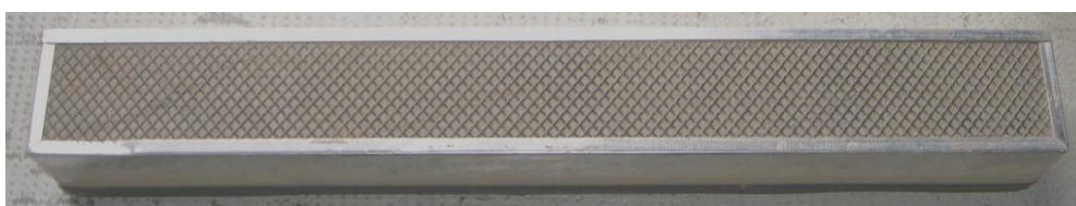
Figure 3: Category 4 filter fitted on the cab prototype.
