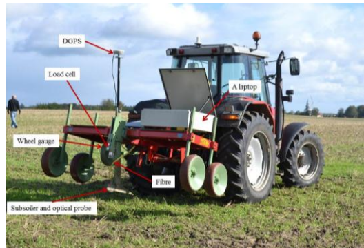
Figure 1: On-line visible and near (vis-NIR) soil sensor (Mouazen, 2006)
